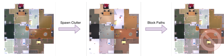
Fig. 3: Example dataset generation process. In this instance, we consider a 10 room floorplan from ProcTHOR-10k. The left image shows the ideal environment without clutter and completely free for optimal navigation throughout the environment. We then generate clutter in the free space using the between-ness centrality of nodes in G_{\text{free}} . The generated obstacle locations are indicated by red circles in the middle image. This causes the blocking of the paths within the accessible rooms, as well as eliminating access to the two rooms on bottom-right of the map, as shown in the right image.
